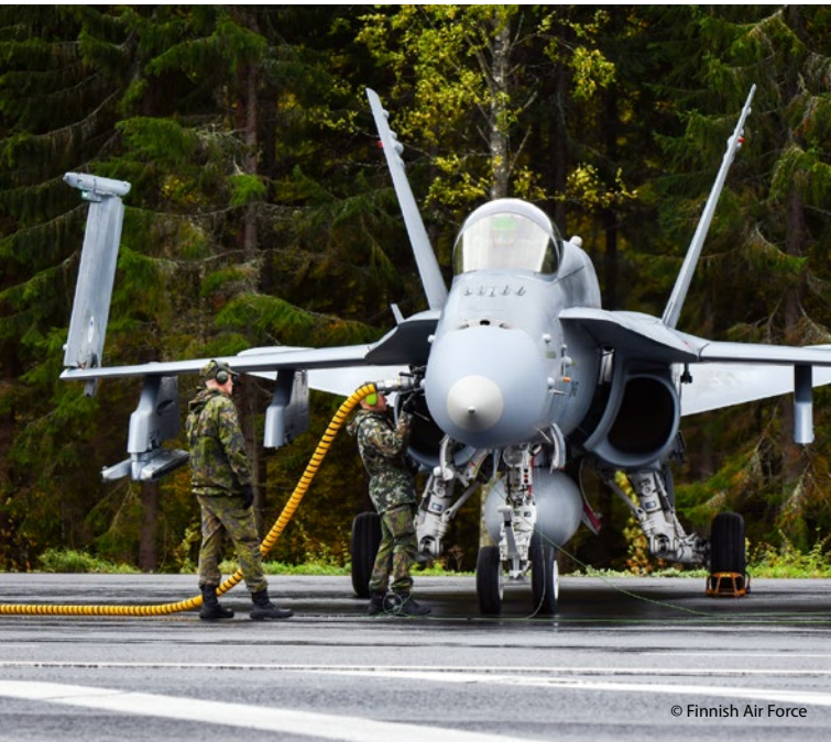
The FINAF ground crew refuelling a Finnish F/A-18 at a road base in Joutsa, showcasing the capability to operate from highway strips.
