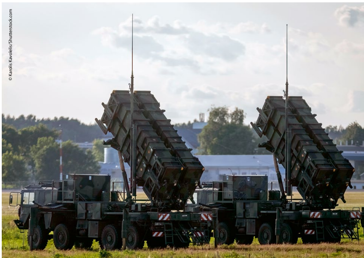
The MIM-104 Patriot Surface-Based Air Defence (SBAD) system is capable of engaging manned and unmanned aircraft, cruise missiles, and tactical ballistic missiles.
